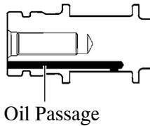
**Cross Section of End of Exhaust Camshaft**
